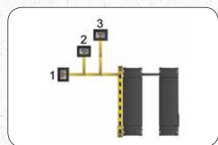
Provided 60" (standard length) air and hydraulic hoses allow three ergonomic, recommended power console placement options.
